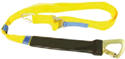
Designed for linesmen climbing wood poles. The KF70126-B is a pole strap / work-positioning device which is clipped to the side 'D's of a harness or work-positioning belt. The adjuster is easy to use one-handed even under tension. A PVC stiffener at the karabiner end allows the strap to be easily passed around the pole before clipping on to the harness 'D' ring.
