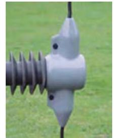
Designed to cover an array of terminals, fittings, conductors and jumpers on overhead powerlines, vermin shrouds prevent flashovers and outages caused by squirrels, birds and other vermin. For use on systems up to 33kV these shrouds are flexible and hard wearing and can be fitted and removed easily. Can be installed by live rubber glove procedures without interruption to the consumer. Please contact us for your individual requirements.
